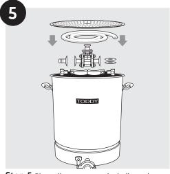
**Step 5** Place all components including valve assembly (Rotate handle on valve to clean ball.), gaskets, hose barb, hose, tri-clamps, and filter platform into bottom of unit below the platform to ensure they are fully submerged.
