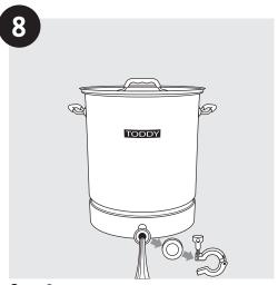
**Step 8** Remove tri-clamp and cleaning blank over sink, drain solution from brewer and allow all parts to air dry *(do not dry with a towel)*.
