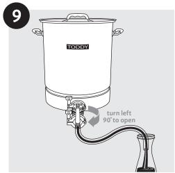
Step 9 Once brewing is complete, place one end of the hose onto the hose barb and the other end into a clean storage vessel. Open valve to drain your cold brew coffee extract. Once draining is complete, refrigerate extract in air-tight containers for up to 2 weeks.
