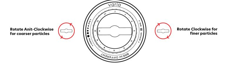
Rotate clockwise until the tightest setting is reached, this position is called the "Start Point".
