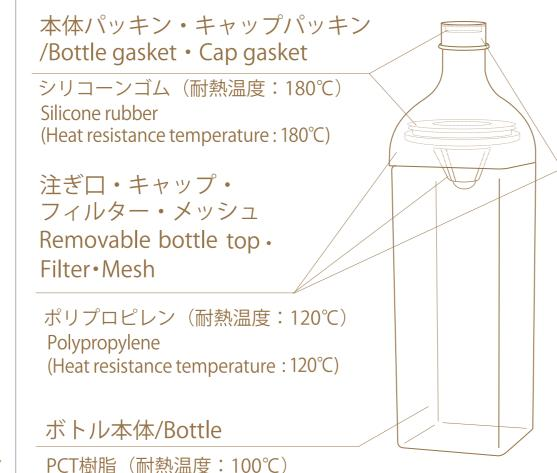
PCT (Heat resistance temperature : 100°C)
