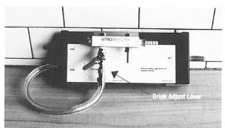
The best starting point for the Nitro Infuser adjustment lever is approximately 10-15% open. This will align with the drink adjust line on the Nitro Infuser label.
