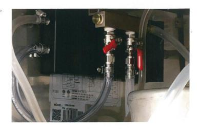
8 b. It will take one or two glasses poured for the coffee to bleed and pressurize the new system. Do not be alarmed if the first glass pours with heavy foam.
